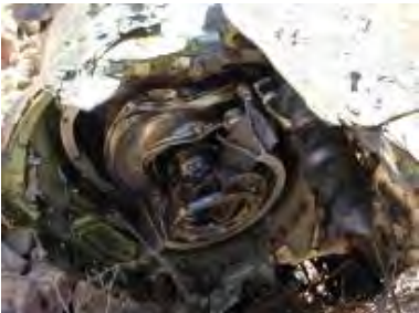
Part of propulsion unit of BGM-109D Tomahawk cruise missile.
