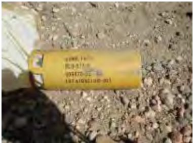
Unexploded BLU 97 cluster bomblet - the Tomahawk BGM-109D cruise missile would have carried 166 of these
