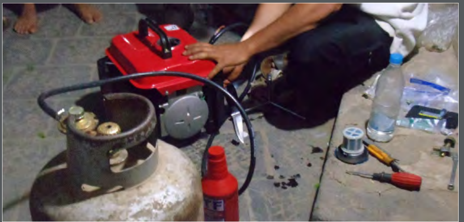
Residents of Old Sana'a have devised methods to run generator using cooking gas amidst the fuel and electricity shortages. Photo by Jeb Boone
