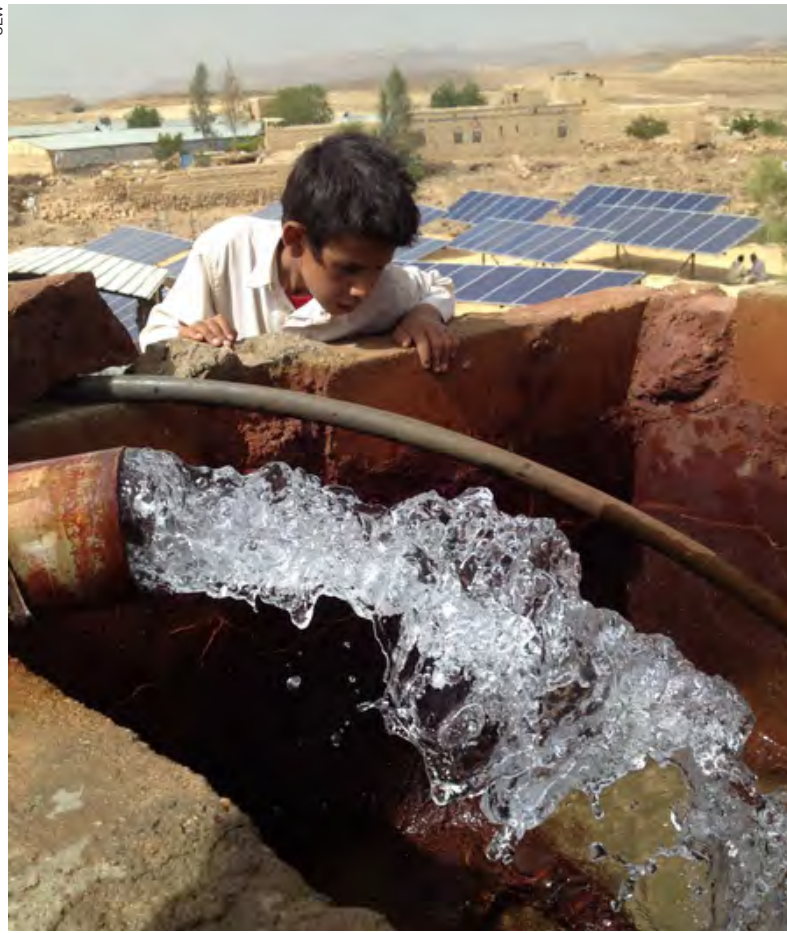
This solar water pump in Al-Safra district of Sa'ada produces 4 liters of water per second.
