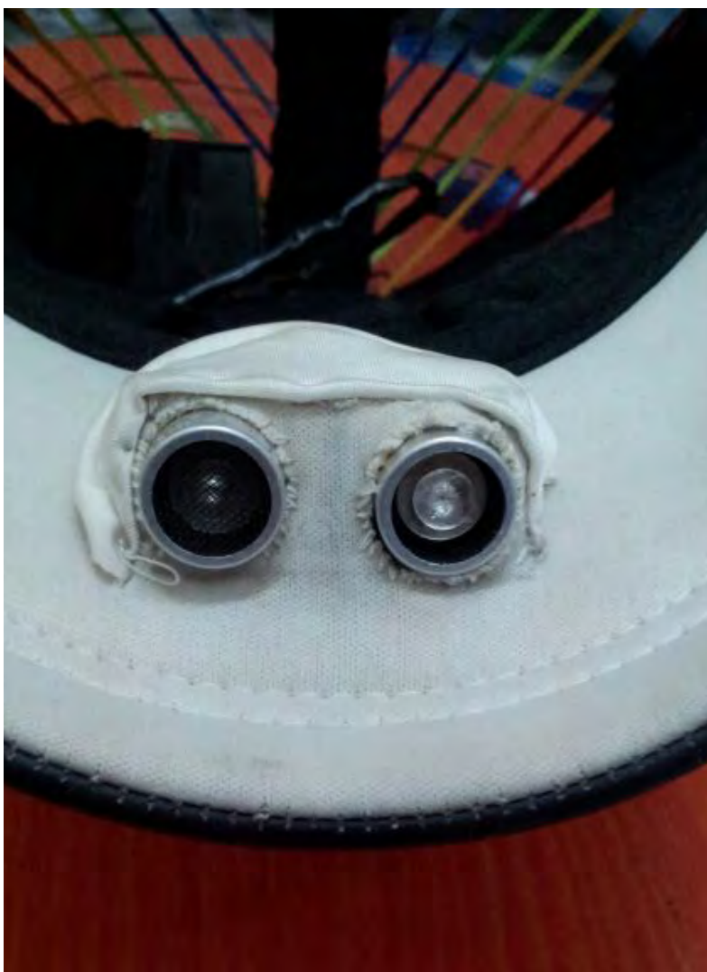
The smart hat uses ultrasounds to help visually impaired sense what is within four meters from them.
