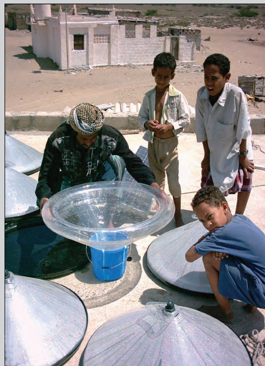
Villagers in Sheikh Salem harvest water from watercones. The product allows individuals to desalinate water on entirely on their own, utilizing condensation and solar irradiation.
