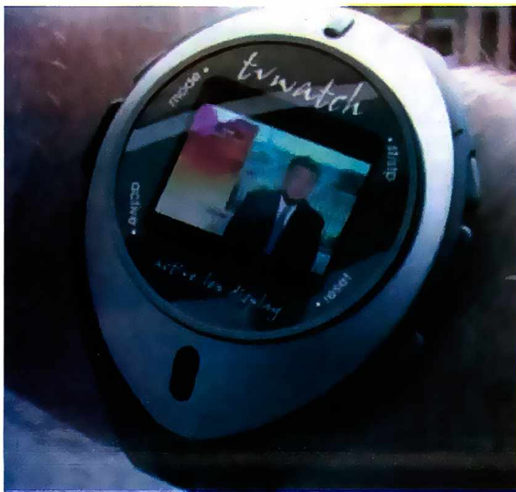
An undated handout photograph shows a Light Emitting Polymer (LEP) TV screen displayed in a wrist watch developed by Cambridge Display Technology, July 19 2002. The watch is one of a range of applications also including roll-up, flexible televisions, which have become possible thanks to a glowing plastic compound perfected in the laboratories of Britain's Cambridge Display Technologies. Photo by Reuters (Handout)
