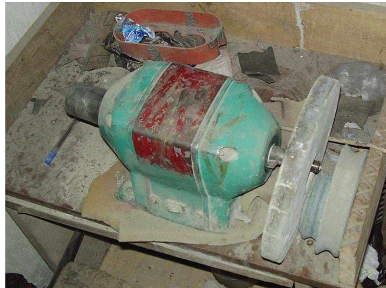
Al-Jalkh, the circular stone that's affixed to the pointed side of the machine. Agates are held to the surface of Al-Jalkh while it rotates to polish them.
