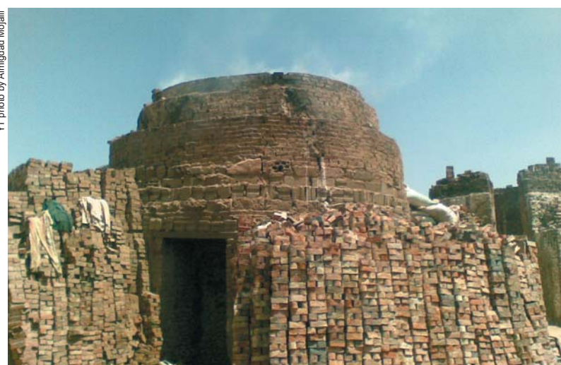
Smoke billows from a brick oven where they are slowly fired to ensure a strong, solid brick.
