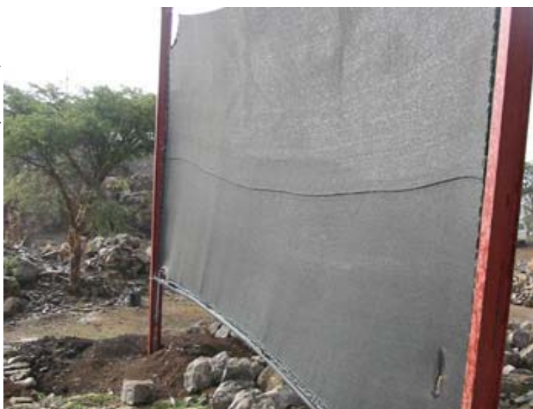
Although expensive, a 40 meter square fog collector can collect up to 180 liters of drinking water from the air in a day.
