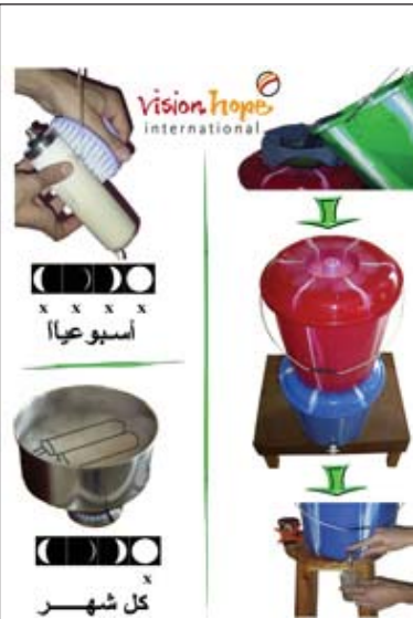
Bucket filters need to be cleaned on a regular basis A VHI chart here explains when according to the moon cycle
