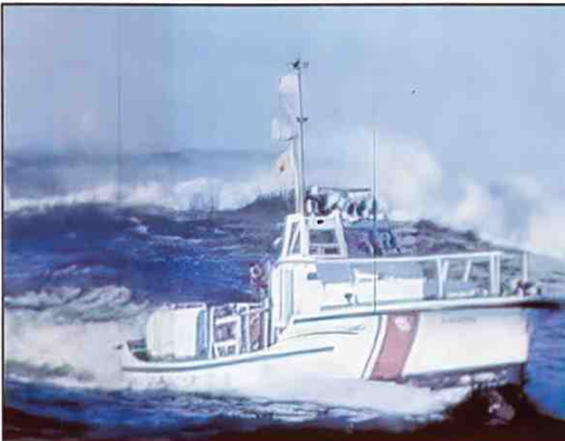
Technical details for the 44 foot motor life boat Length:13.62m Beam: 3.84m Displacement approx. 18.5tons Speed: 15.5 knots Range:190 nautical miles Crew:5 First built:1964, last built: 1982 Designed by the US coast guard
