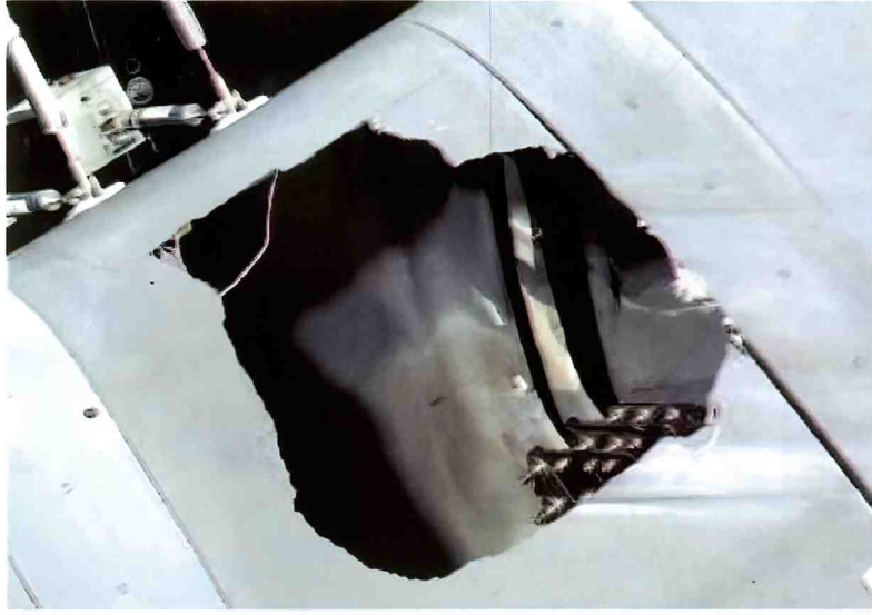
File photo shows a 16-inch hole in a carbon-reinforced wing panel removed from shuttle Atlantis after a 1.67-pound piece of fuel-tank foam insulation was shot out of a 35-foot nitrogen-pressurized gun and slammed into it during a test. The final report on the space shuttle Columbia disaster, released on Tuesday, said NASA's self-protective culture and its reluctance to tackle safety problems head-on contributed to the fatal breakup of shuttle Columbia that killed seven astronauts. REUTERS
