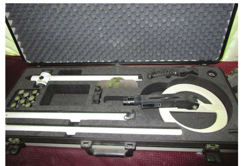
A device used by YEMAC's technical team to detect mine-infected areas.
